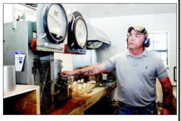
Staff Sgt. James Taylor, WTB, tests the strength of a concrete sample at the Corps of Engineers Quality Assurance Office at Fort Hood. Taylor has been with the agency for more than four months.
